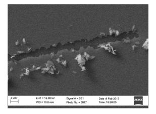
**Fig. 4.** Specifics of the structure of the crystalline  $ScGe_2$  thin film after long aging (X3000).
