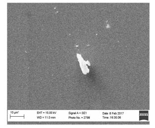
Fig. 2. Electron micrograph of crystalline LaNiGe<sub>2</sub> thin films, obtained by discrete evaporation at  $v_p = 5$  nm/sec and  $T_p = 700$  K, after 20 years of aging (X1000).
