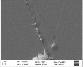
**Fig. 3.** The repercussion of recrystallization processes during the long aging in crystalline LaFeGe<sub>2</sub> condensate (X2000).
