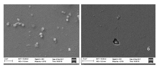
Fig. 1. Morphology of  $Y_{25}Fe_{25}Ge_{50}$  thin films, obtained by  $v_p = 6$  nm/sec and  $T_p = 710$  K by coevaporation, after long aging in desiccator (a - X6000; b - X2000; the scale in the left corner micrographs is shown).
