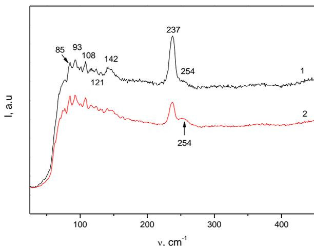
**Fig. 4.** Raman spectra of  $\text{Se}_{97}\text{Sb}_3$  (1) and  $\text{Se}_{93}\text{Sb}_7$  (2) films measured at a laser radiation power of 10 mW.
