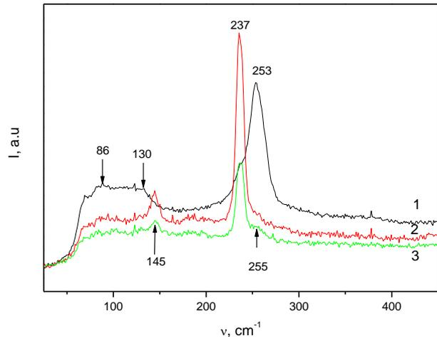
**Fig. 3.** Raman spectra of  $\text{Se}_{93}\text{Sb}_7$  films, nominally pure (curve 1) and modified with mercury during 48 (curve 2) and 120 (curve 3) hours.
