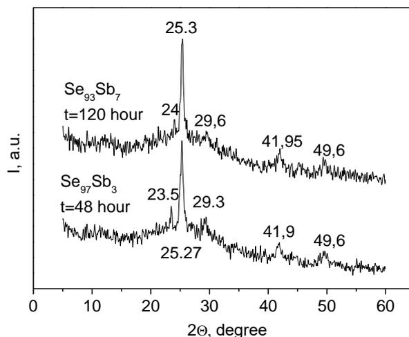
**Fig. 1.** X-ray diffractograms of amorphous  $\text{Se}_{97}\text{Sb}_3$  and  $\text{Se}_{93}\text{Sb}_7$  films, exposed in mercury vapor for 48 and 120 hours, respectively.
