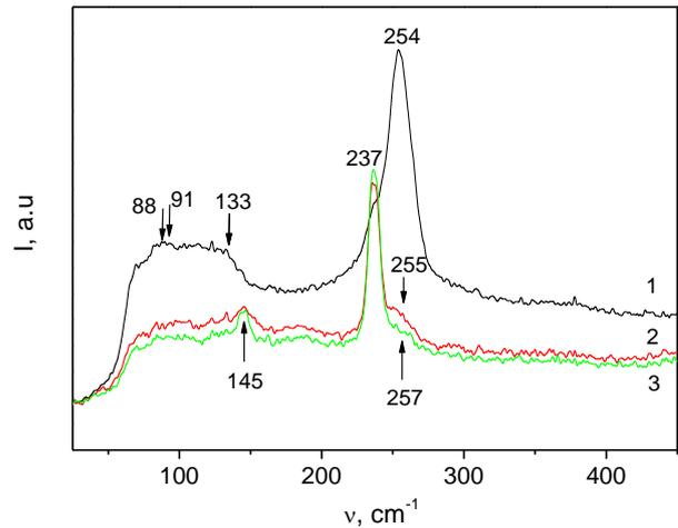
**Fig. 2.** Raman spectra of nominally pure (curve 1) and mercury-modified  $\text{Se}_{97}\text{Sb}_3$  films for 48 hours (curve 2) and 120 (curve 3) hours.
