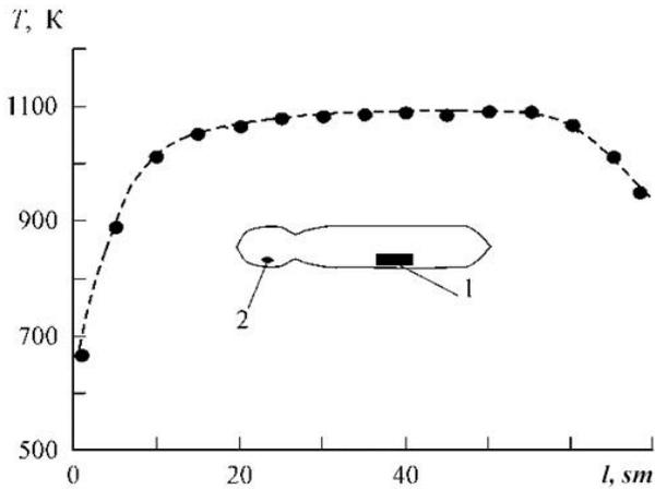
**Fig. 1.** Temperature distribution and position of ampoules when obtaining diffusion layers: 1 – substrate of the starting material; 2 – the sample.
