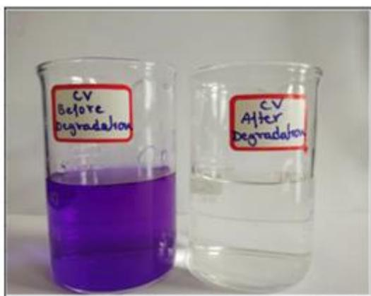
Fig. 27. Results of photodegradation of crystal violet [47].
