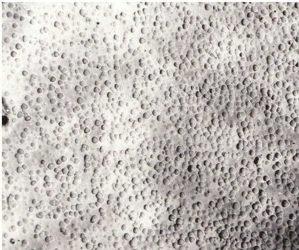
**Fig. 2.** The surface of the YIG film etched by PbO vapor, zoom: x200.
