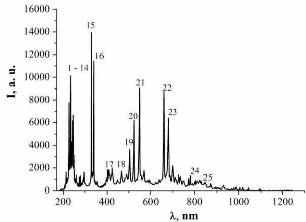
**Fig. 5.** The radiation spectrum of a nanosecond discharge between the electrodes of the  $Ag_2S$  compound at the atmospheric pressure of Nitrogen and the frequency  $f = 1000$  Hz.
