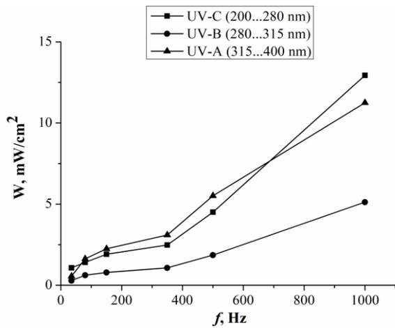
**Fig. 2.** Dependencies of UV power density – radiation in the UV-C, UV-B, UV-A ranges for the discharge plasma on the frequency of repetition of voltage pulses at a charging voltage of  $U = 13$  kV in Nitrogen between electrodes with  $Ag_2S$  at a pressure of  $p(N_2) = 101$  kPa.
