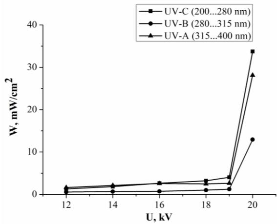
**Fig. 3.** Dependencies of UV power density - UV-C, UV-B, UV-A radiation - discharge ranges on the voltage on the electrodes at  $f = 80$  Hz in atmospheric pressure nitrogen between  $Ag_2S$  electrodes.
