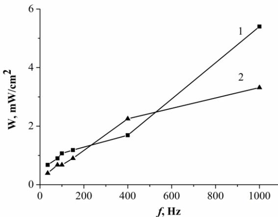
**Fig. 4.** Dependencies of UV power density – UV-A radiation – discharge range on the frequency of repetition of current pulses at a charging voltage of  $U = 13$  kV in atmospheric pressure nitrogen between electrodes with  $Ag_2S$  at pressures: 1 – 101 kPa and 2 – 13.3 kPa.
