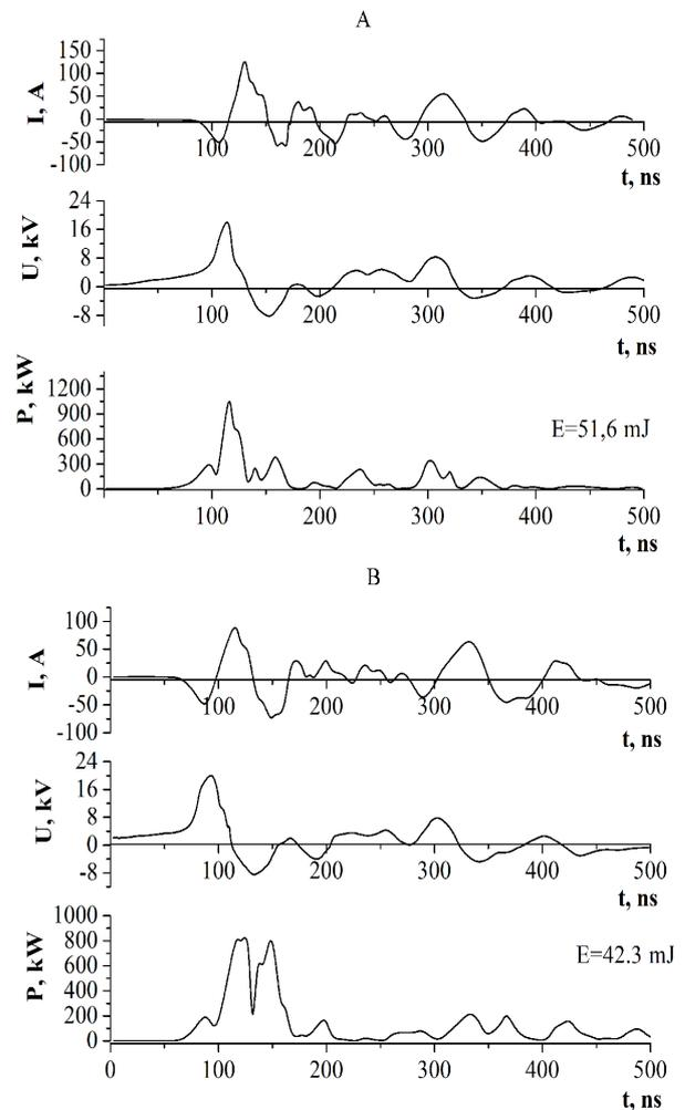
**Fig. 1.** Oscillograms of current pulses, voltages, pulsed power, and energy contribution to the plasma of an overvoltage nanosecond discharge for one discharge pulse ( $p(\text{N}_2) = 101$  kPa, (A); 13.3 kPa (B)).
