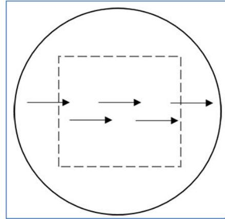
Fig. 1 Surface roughness path taken across disc.
