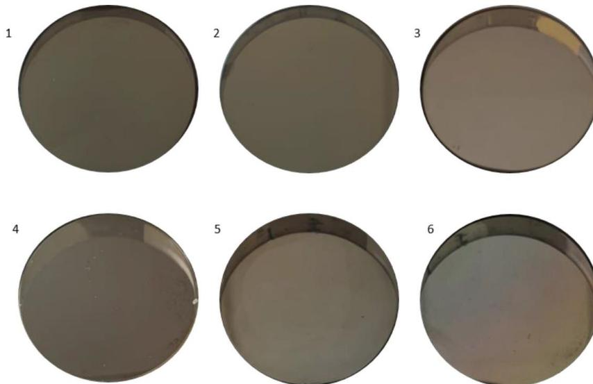
**Fig. 6** Discs after 2.5 Mc of testing: CoCrMo discs number 1,2,3 with titanium interlayer under DLC after 2.5 Mc of testing; CoCrMo discs number 1,2,3 without titanium interlayer under DLC after 2.5 Mc of testing.
