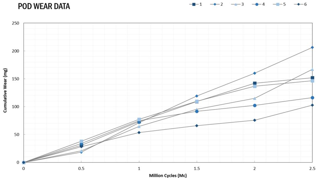
**Fig.3** Cumulative wear of PE pins during 2.5 Mc POD test.
