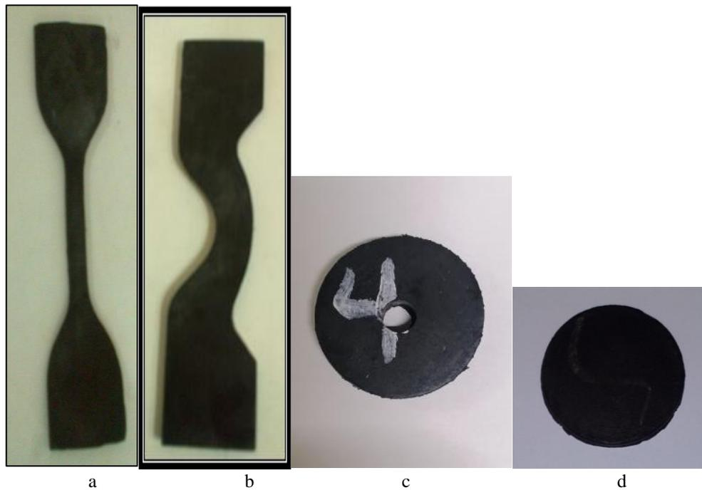
**Fig. 2.** Samples for tests: a. Tensile test (ASTM D412), b. Tear Test (ASTM 624), c- Hardness and resilience tests (ASTM D7121), d- Abrasion test (ASTM 2228).
