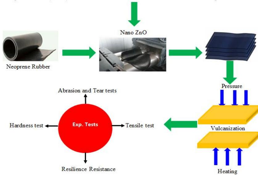
**Fig. 1.** The preparation process of Neoprene rubber composites and experimental tests.
