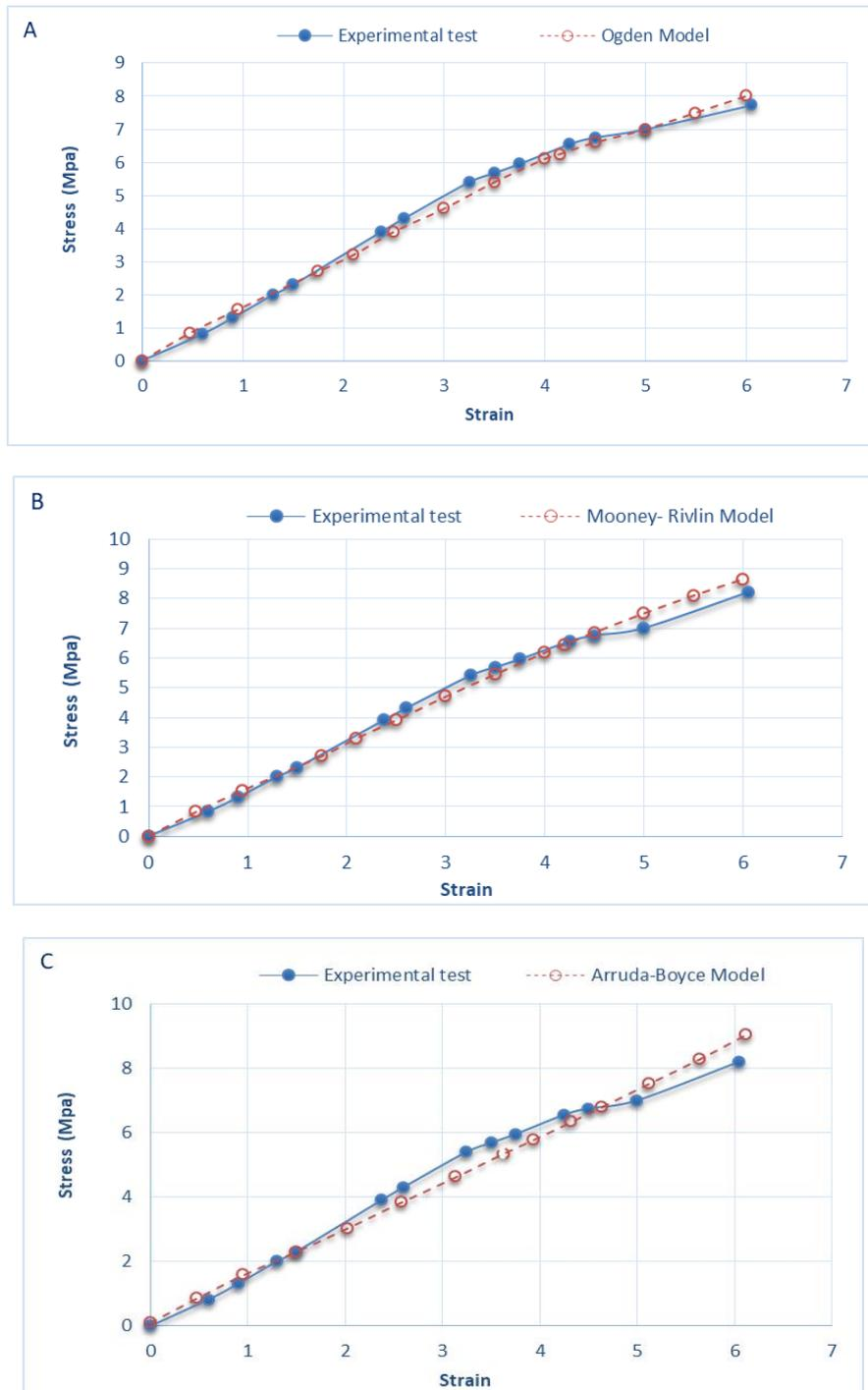
**Fig. 5.** Stress-Strain curve of 2.4 % ZnO PHR with four hyperelastic models: A) Ogden model, B) Mooney-Rivlin model, C) Arruda-Boyce model.
