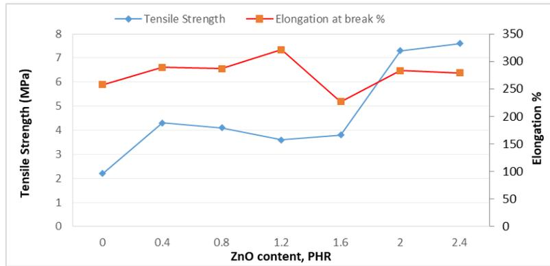
Fig. 3. Effect of Nano ZnO content on CR/NR composites tensile strength and ductility samples.
