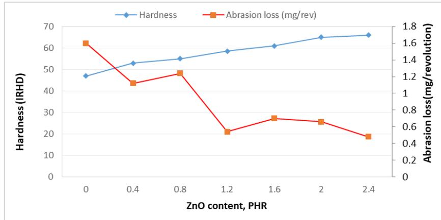
Fig. 4. Effect of Nano ZnO content on CR/NR composite hardness and abrasion loss samples.
