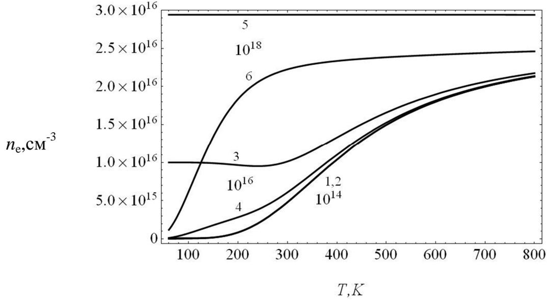
**Fig. 3.** Temperature dependence of concentration of ground state electrons for the 3D CQDS InAs/Ga<sub>0.15</sub>In<sub>0.85</sub>As ( $L = 96 \text{ \AA}$ ) at different impurity concentrations (curves 1,2 refer to  $10^{14} \text{ cm}^{-3}$ ; curves 3,4 stand for  $10^{16} \text{ cm}^{-3}$ ; curves 5,6 relate to  $10^{18} \text{ cm}^{-3}$ ) and energies of occurrence of the impurity level (curves 1,3,5 refer to  $-150 \text{ meV}$ ; curves 2,4,6 stand for  $-750 \text{ meV}$ ).
