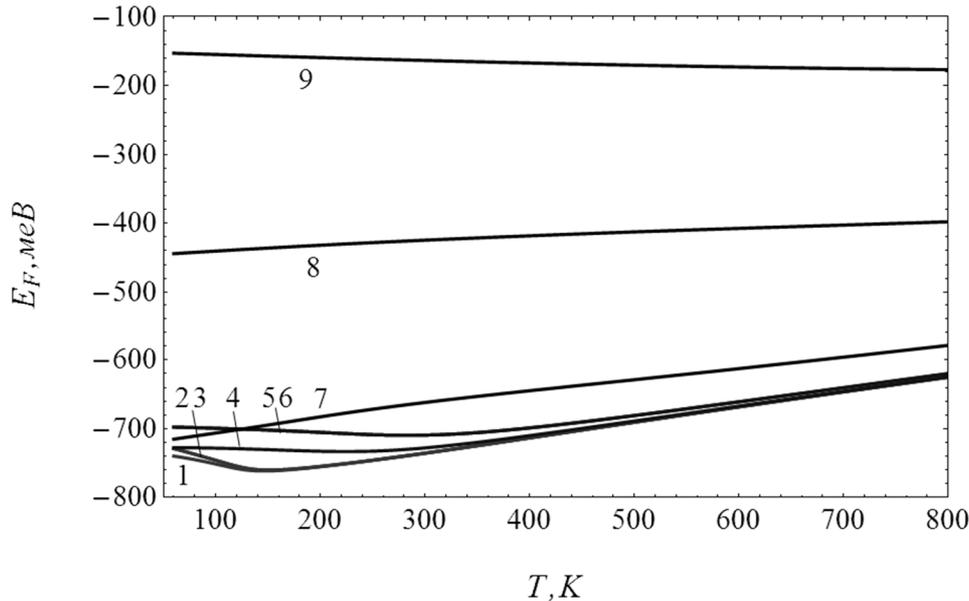
**Fig. 2.** Temperature dependence of the Fermi energy of the 3D InAs/GaAs CQDS ( $L=96 \text{ \AA}$ ) at different concentrations of impurities (curves 1,2,3 refer to  $10^{14} \text{ cm}^{-3}$ ; curves 4,5,6 relate to  $10^{16} \text{ cm}^{-3}$ ; curves 7,8,9 refer to  $10^{18} \text{ cm}^{-3}$ ) and energies of occurrence of the impurity level (curves 1,4,7 attribute to  $-750 \text{ meV}$ ; curves 2,5,8 refer to  $-450 \text{ meV}$ ; curves 3,6,9 relate to  $-150 \text{ meV}$ ).
