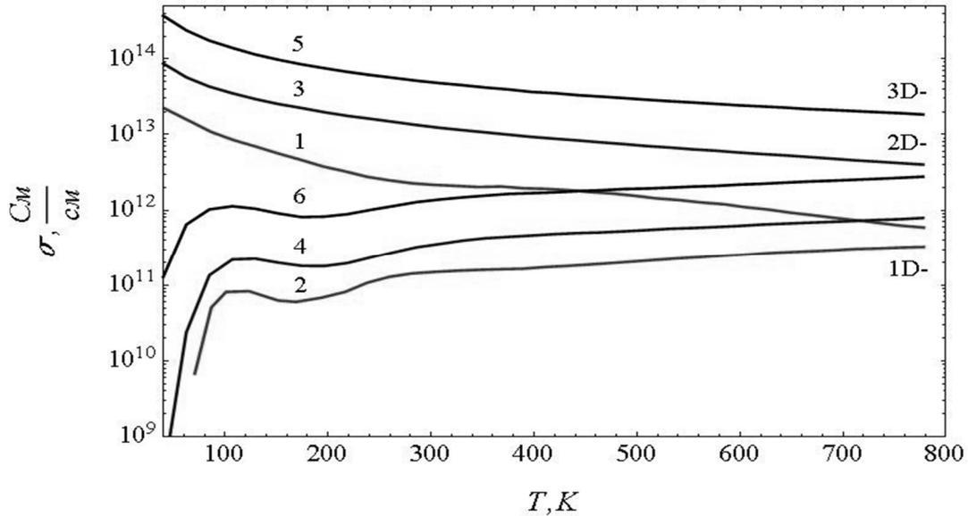
**Fig. 4.** Temperature dependence of electroconductivity of the InAs/Ga<sub>0.15</sub>In<sub>0.85</sub>As ( $L=96 \text{ \AA}$ ) CQDS of various dimensionality (curves 1,2 stand for 1D; curves 3,4 refer to 2D; curves 5,6 relate to 3D), energies of occurrence of the impurity level  $E_D$  (curves 1,3,5 refer to  $-150 \text{ meV}$ ; curves 2,4,6 stand for  $-750 \text{ meV}$ ) at concentration of impurities  $10^{18} \text{ cm}^{-3}$ .
