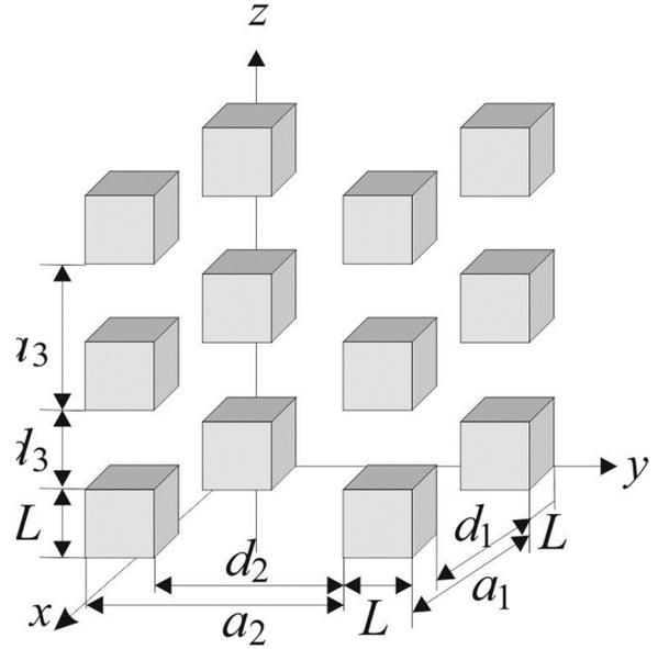
**Fig.1.** Geometry of the cubic quantum dot superlattice.
