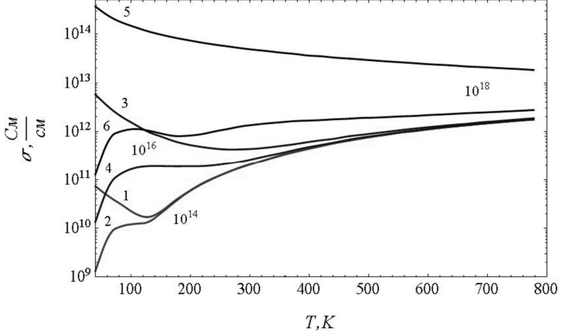
**Fig. 5.** Temperature dependence of electroconductivity of the 3D InAs/Ga<sub>0.15</sub>In<sub>0.85</sub>As ( $L=96$  Å) CQDS at different concentrations of impurities:  $10^{14}$  cm<sup>-3</sup> (curves 1,2);  $10^{16}$  cm<sup>-3</sup> (curves 3,4);  $10^{18}$  cm<sup>-3</sup> (curves 5,6) and energies of occurrence of the impurity level (curves 1,3,5 refer to -150 meV; curves 2,4,6 stand for -750 meV).
