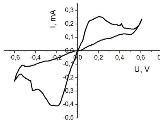
**Fig. 9.** Cyclic voltamperogram of  $\text{Ag}/\text{Ag}_8\text{SnSe}_6/\text{C}$  cell.
