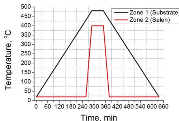
**Fig. 2.** Temperature profiles of  $\text{Ag}_8\text{SnSe}_6$  synthesis by selenization method.
