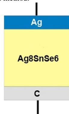
**Fig. 3.** Scheme of solid electrochemical cell  $\text{Ag}/\text{Ag}_8\text{SnSe}_6/\text{C}$ .
