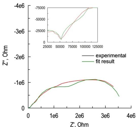
**Fig. 6.** Experimental and modeled Nyquist plot for the  $\text{Ag}/\text{Ag}_8\text{SnSe}_6/\text{C}$  cell. On insert presented high-frequency part of plot. The values of real ( $Z'$ ) and imaginary ( $Z''$ ) part of impedance given in Ohms.
