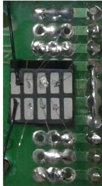
Fig. 4.  $\text{Ag}/\text{Ag}_8\text{SnSe}_6/\text{C}$  resistive switching cell.
