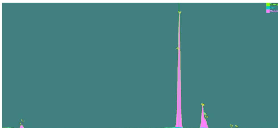
**Fig. 1.** Energy dispersive X-ray spectrum of Ag-Sn target.
