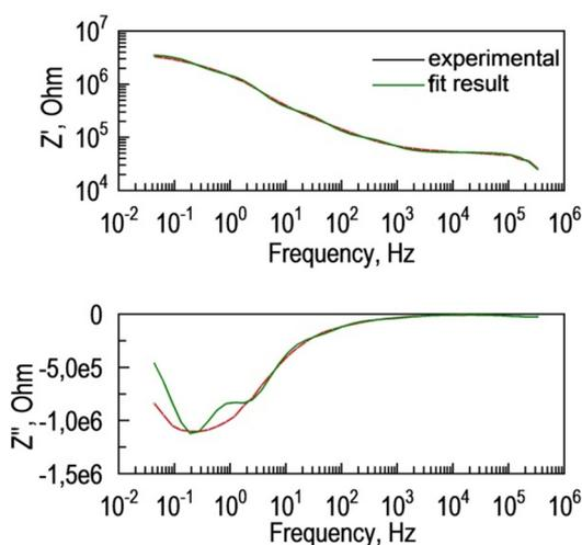
**Fig. 7.** Experimental and modeled Bode plot for the  $\text{Ag}/\text{Ag}_8\text{SnSe}_6/\text{C}$  cell. The values of real ( $Z'$ ) and imaginary ( $Z''$ ) part of impedance given in Ohms.
