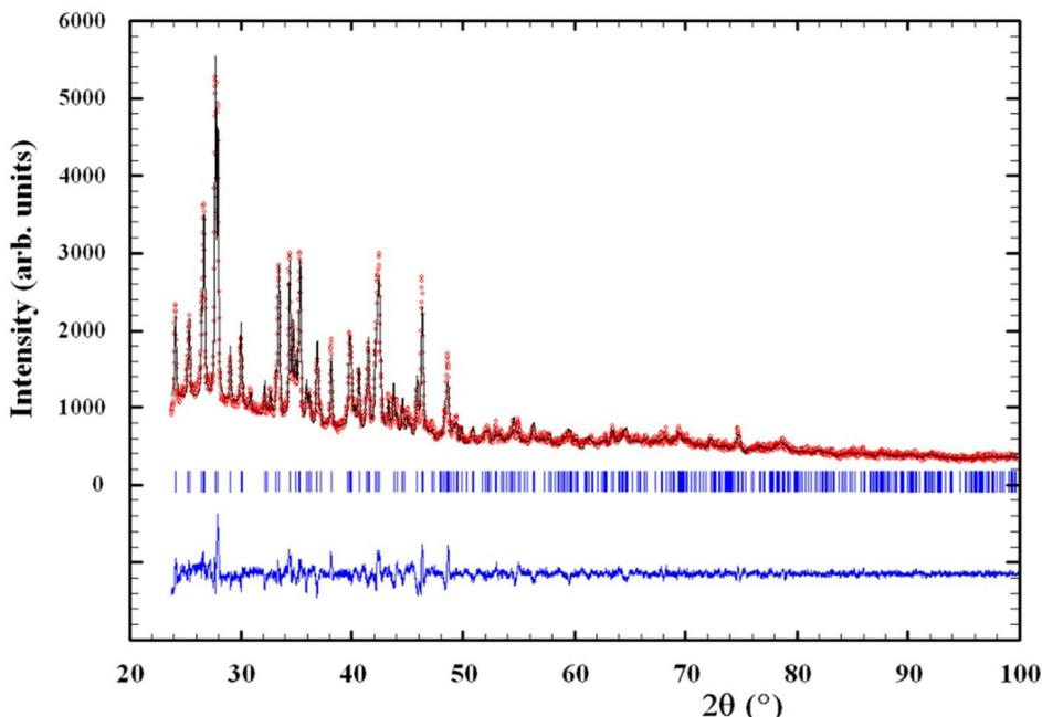
Fig. 5. X-ray diffractogram of synthesized  $\text{Ag}_8\text{SnSe}_6$  argyrodite thin film.
