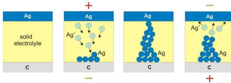
**Fig. 10.** Scheme of resistive switching process in solid state cells.
