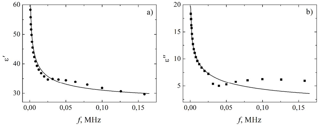
**Fig. 2.** Frequency dependences of the effective values of the permittivity  $\epsilon'(f)$  and  $\epsilon''(f)$  components for  $H_xGaSe$  single crystals (sample 2).
