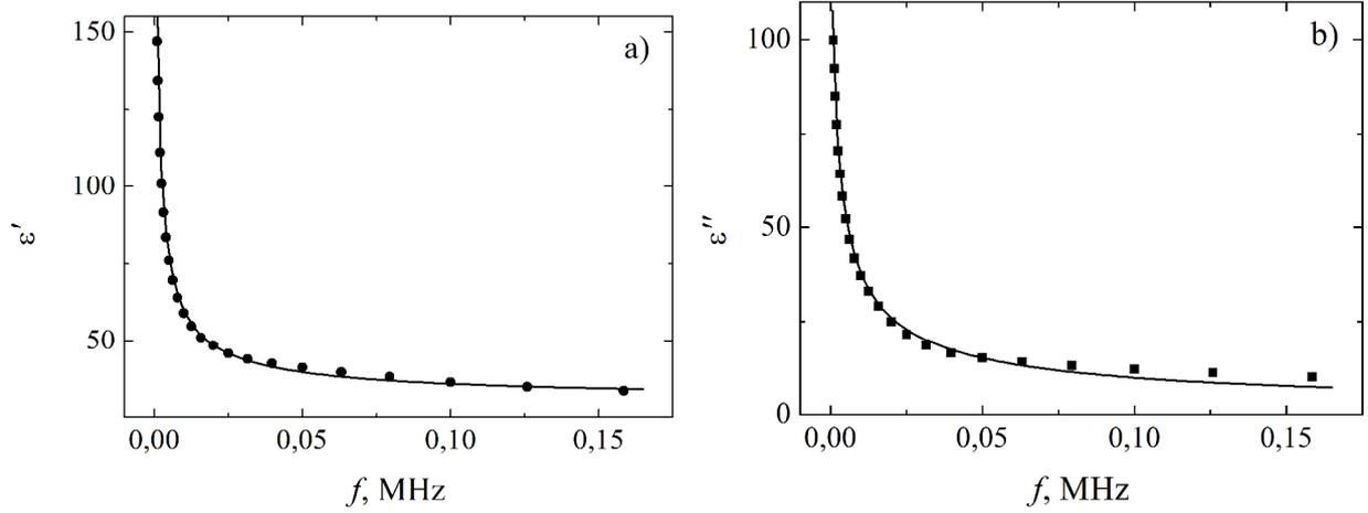
**Fig. 1.** Frequency dependences of the effective values of the permittivity  $\epsilon'(f)$  and  $\epsilon''(f)$  components for  $H_xGaSe$  single crystals (sample 1).
